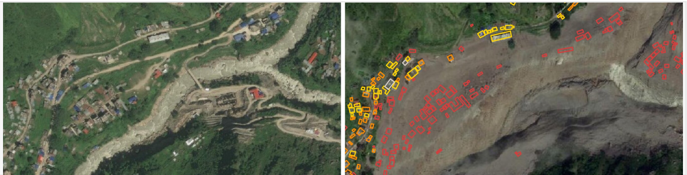
Syaphrubesi, before (Vantor, Sep 2023) and after, with fAIr damage classes: red destroyed, orange major, yellow minor.
