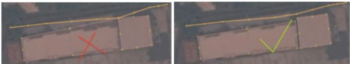
(Left) Building and road are connected and (right) building and road are separated
